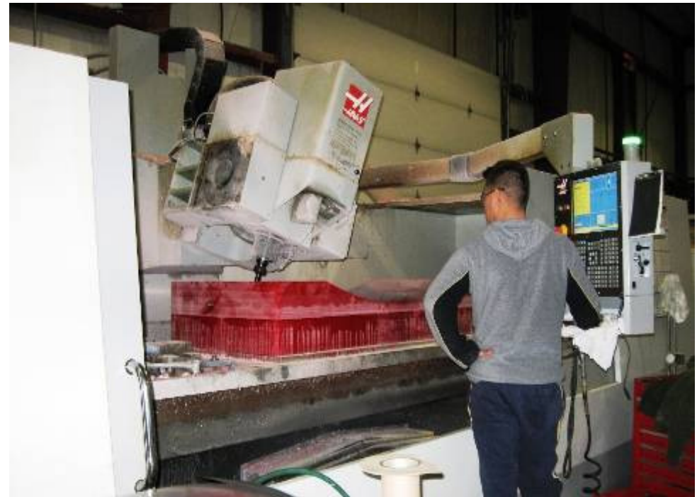
HAAS VR11 5 Axis CNC MC Table 120" x 40"
